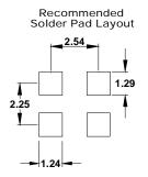
Note: XPRESSO HCMOS XOs are designed to fit on industry standard, 4 pad, layouts.
