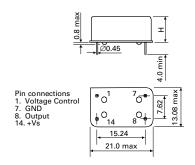
Frequency Range 1.0 to <30.0MHz 30.0 to 90.0MHz Height (H) 5.1 max. 8.0 max.
