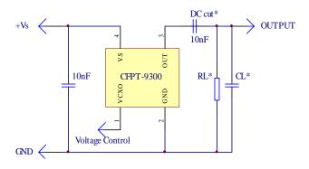
\*DC cut capacitor required for AC coupled Clipped sinewave.
