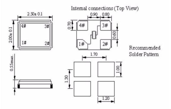
Holder Style Mode Adjustment Tolerance Temperature Stability Operating Temp. Range Load Capacitance ESR Ageing Marking 25x2x05 4-pad Fundamental ± 10PPM at 25°C ± 15 PPM -30°C to +85°C 16 pF 150 Ohm +/-1ppm AEL16
