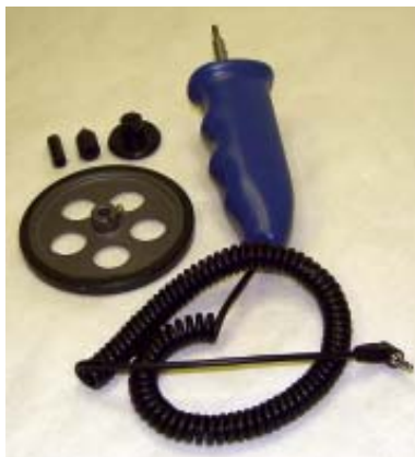
Remote Magnetic Sensor (MT-190-P) Gap 0.25 inches
