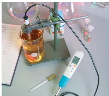
testo 206-pH3 facilitates the connection of external pH probes
