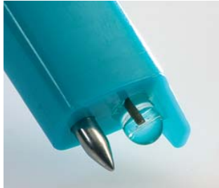
pH1 probe head for liquids
