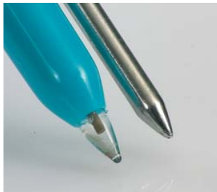
pH2 probe head for semi-solid substances
