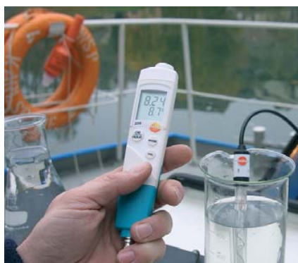
Automatic temperature compensation in external probes with temperature sensor
