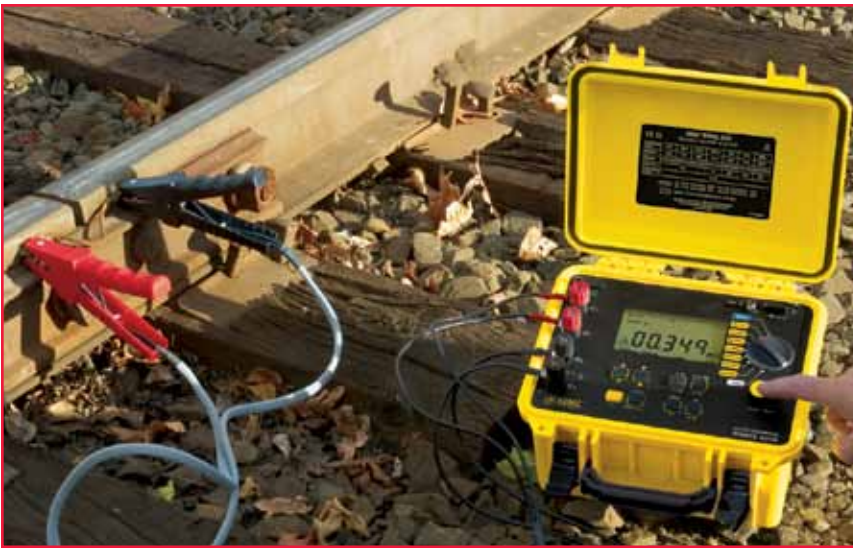
Verifying rail bonds with the Model 6250
