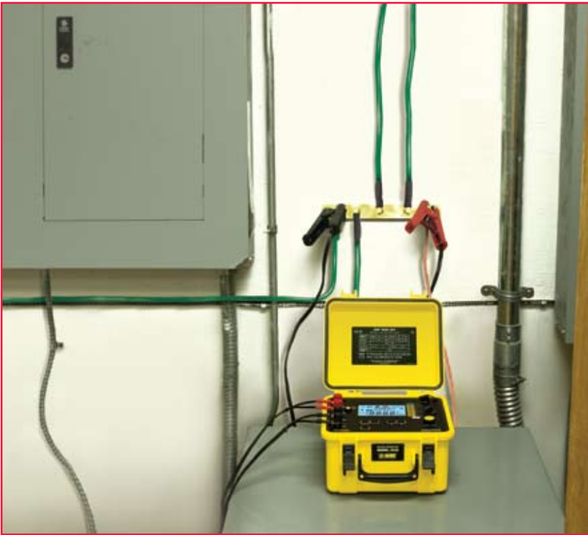
Model 6240 checks contact resistance on a ground bus.
