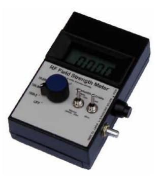
comparison, a typical cordless phone will produce about  $0.01~\mu\text{W/cm}^2$  at a distance of 50 feet. At FM, TV and mobile phone frequencies, accuracy, is better than 3dB. Unlike many other power meters, it has built-in antenna and detection system which yields a flat response over a very wide range of frequencies. Even at 5GHz, signals can still be measured. The meter features an internal 9v battery with a low battery indication when there is about 10 minutes life remaining.
