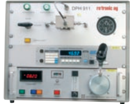
DPH 911 Reference dew point mirror for certification of SCS* humidity standards
