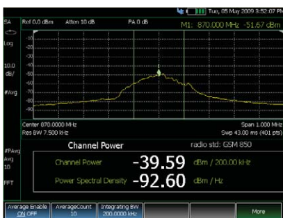
Channel power measurement
