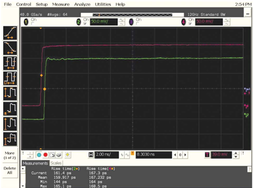
Figure 4 Time domain differential probe response, purple = input of the probe, green = probe output, using Agilent 1169A InfiniiMax probe and DS081304B 13 GHz oscilloscope
