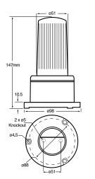
The FFA125 Series operates through an internal circuit which simply cycles the lamp On and Off. These type of beacons generally give a much lower light output as it takes longer for the lamp to fully illuminate itself. These units are available with a
