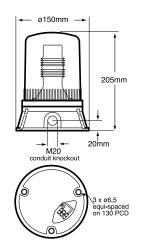
The FF401/400 Series operates through an internal circuit which simply cycles the lamp On and Off. These type of beacons generally give a much lower light output as it takes longer for the lamp to fully illuminate itself. These units are available with either a filament or tungsten halogen lamp. The light
