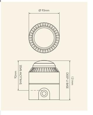
The Flashni is an audible and visual device which requires one single installation point. This greatly reduces installation and costs and is much less obtrusive than two separate devices. Versions are available with the sounder and beacon linked, or with separate terminals for independent operation.
