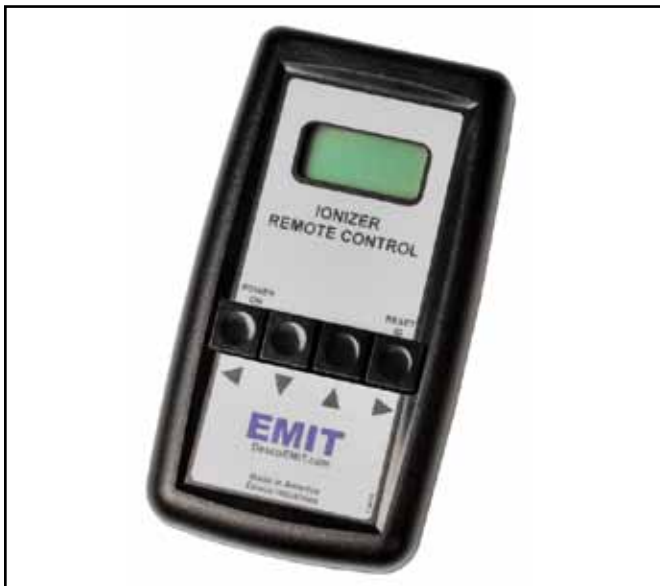
Figure 1. Infrared Remote Control
