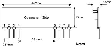
Pins on 0.1" pitch Pin Dims :0.6 x 0.6mm
