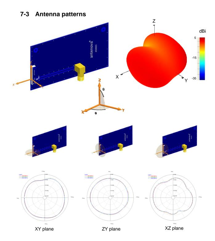
Patterns show combined polarisations measured on reference board A5660
