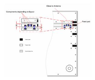
Antenna feed pad indicated. All other pads should be connected to ground.
