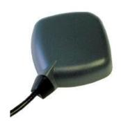
The WS3917 GPS antenna is a high value antenna with a wide voltage range, ideally suited to AVL and telematics platforms for vehicle-mounted use. Using internal magnets or screw mount holes, the antenna can be installed almost anywhere on a vehicle allowing great flexibility. The WS3917 antenna features a high gain (28 dB) low noise amplifier and a SAW filter. With a wide range of connectors and 2.7 to 5 volt operation, the antenna can be used with almost any GPS system available.
