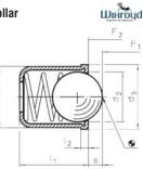
Material Body: stainless steel 1.4305 or Delrin blue. Ball: stainless steel, hardened or Delrin white (POM). Spring: stainless steel. Technical Notes Used for locating, applying pressure or lifting off. spring loads \* = statistical average values.
