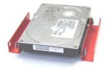
HDD mounting brackets for both 3.5in and 2.5in HDD. Can be used for mounting HDD in either horizontal or vertical position. By using 8 dampers it can protect in XYZ directions. The Kit includes dampers and screws.
