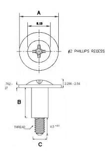
A one piece-fixing bolt can replace a three-part assembly of screw, washer and tube. Designed to give optimum Compression to the GVD range of dampers. The threads are suitable for screwing directly into a HDD. Available in UNC 6-32 or M3 thread.
