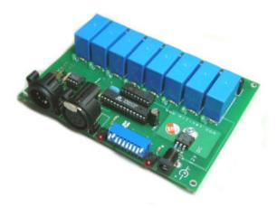
The DMX Relay board provides up to 8 digital outputs when connected to a DMX theatre control network. The base address may be set to between 1 and 505. Ordering options include a custom case and provision for solid state relays.
