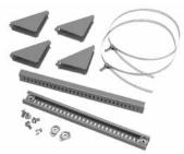
Use to mount CONCEPT<sup>®</sup>, Networking and wall-mount enclosures to poles of various sizes and shapes. Simply attach the plated steel channel bar to the mounting holes at the back of the enclosure and wrap the stainless steel strap around the pole and through the bar. Kit includes two mounting channels, two straps suitable for 3-in. (76mm) to 12-in. (305-mm) diameter pole and mounting hardware. Bulletin: CWY
