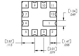
TOLERANCE IS ±.005 [ 0.13 ] DIMENSIONS ARE IN INCHES AND [MILLIMETERS].
