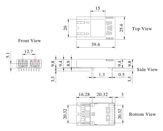
All dimensions are in millimeters (mm)
