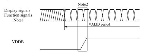
Note1: These are the display and function signals for LCD panel signal processing board.
