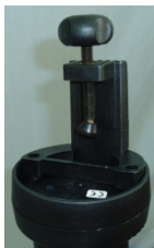
Clamp Fitted to Base
