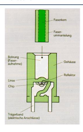
Easy coupling Standard POF 2,2 mm Diameter 1 mm Corediameter
