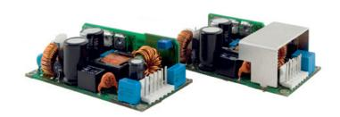
The new TOP-100 Series AC/DC Power Supplies feature the highest power rating in the industry standard  $2.0'' \times 4.0''$  (50.8 x 101.6 mm) footprint. They can supply up to 100 W output power with convection cooling over an industrial operating temperature range of -25 °C to +50 °C. This performance could be realized by a state of the art design providing an extremely high efficiency of >90 % which eliminates the need for a dedicated power supply cooling fan.
