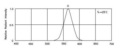
wavelength  $\nearrow$  (nm) RELATIVE INTENSITY Vs. WAVELENGTH
