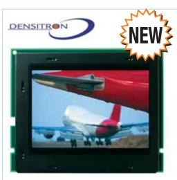
Densitron has come up with another innovative LCD product: a 320 x 234 dot, 32K colour, 5V operation, 8051 bus interface TFT LCD for all low-to-mid volume industrial applications.
