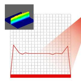
Applications are mainly in the image processing industry for the light-section method.
