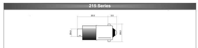
Dimensions in mm (Typical) Not to Scale Green dot on base of product indicates centre contact cathode -ve. Colour dot on sleeve denotes LED colour.
