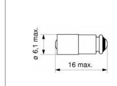
Part Number: 1512145W3D Serial Number: 15121 Based LED type: StarLED Size (inch): T-1 3/4 Size (mm): T6
