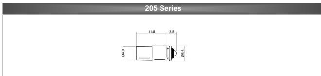
Dimensions in mm (Typical) Not to Scale Green dot on base of product signifies reverse polarity. Colour dot on LED denotes LED colour.
