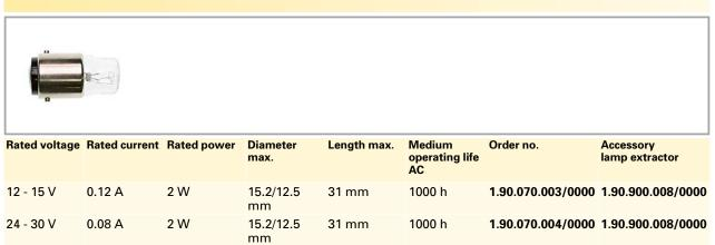
Ratings and operating life specifications generally refer to the lower rated voltage value. Operating life specifications of lamps refer to AC operation. With DC operation, these are reduced by about 40%.
