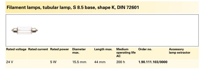
Ratings and operating life specifications generally refer to the lower rated voltage value. Operating life specifications of lamps refer to AC operation. With DC operation, these are reduced by about 40%.
