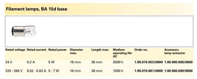
Ratings and operating life specifications generally refer to the lower rated voltage value. Operating life specifications of lamps refer to AC operation. With DC operation, these are reduced by about 40%.
