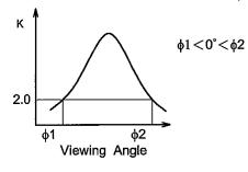
Contrast ratio K vs viewing angle  $\phi$
