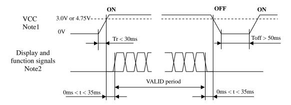
Note1: In terms of voltage variation (voltage drop) while VCC rising edge is below 3.0V in "VCC = 3.3V" or 4.75V in "VCC = 5.0V", a protection circuit may work, and then this product may not work.
