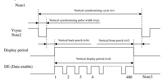
Note1: This diagram indicates virtual signal for set up to timing.
