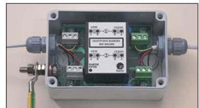
ESP 30D/2BX with lid removed to show internal connections. Note the colour coded, grey and green, terminals
