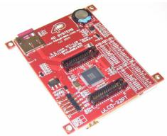
The serial platform allows users to develop their application using their favourite micro-controller and software development tools. In short, the uLCD-32PT(SGC) display module offers some of the most flexible embedded graphics solutions available.
