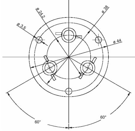
The outer geometry of all the Tri-lenses (Narrow, Medium and Wide beam) are the same for the different beams, except the top of the lens. The lens can be identified by the top view:
