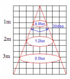
These values have been calculated using the efficiency values of the lens listed above and the formula  $E = I / d^2$ , where E is the irradiance in lux, I the intensity in cd, and d the distance between the lens output and the measured point.
