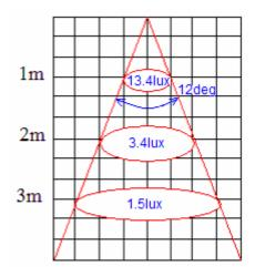
With FLP-HMB3-LL01-0 lens: Low Profile Medium Beam lens for Lambertian Luxeon LEDs
