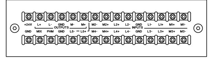
**AUDIO INPUTS:** Inputs are labeled **1** through **5.**, **L** is for line level inputs, **M** is for mic level inputs. You may use either the mic or line terminals for inputs 1-4, Input 5 is line only. Both may not be used simultaneously. Connect balanced audio to **+**, **-**, and ground. Connect unbalanced audio to **+** terminal; connect **-** to ground terminal together with the unbalanced shield.
