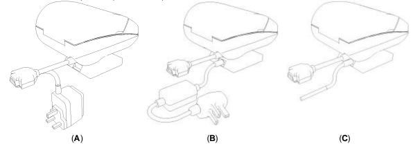
All three options are housed in the same type of replaceable pack, which clips into the underside of the printer and can be changed in a few seconds by the user. In each case, the primary power for the printer comes from this replaceable pack.
