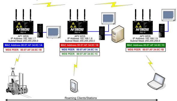
The 702-Ws have been configured as peers. This allows forklifts or other mobile wireless device to maintain communication as they move from the area covered by one 702-W into the area covered by the next 702-W.
