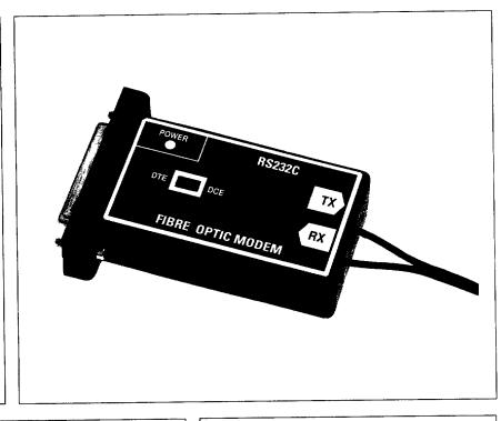
The GO232 is a low cost, full duplex to 19200 baud fibre optic RS-232 modem. Supporting software handshakes (Xon/Xoff), utilising up to 100 metres of twin core 1mm plastic fibre (Eska Extra 4002 or equivalent). To make the fibre connection, simply cut the fibres to the length required using side cutters or a knife. Insert fibres into GO232 and tighten locking screw.
