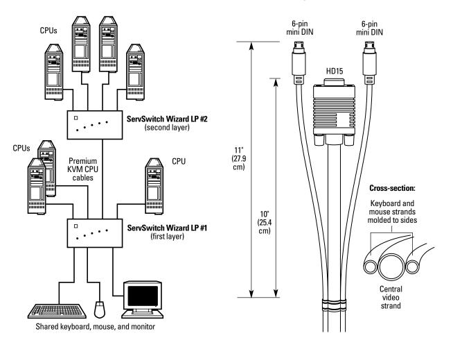
The ServSwitch Wizard LP (4-port model shown here) packs a ton of useful components into the least possible space.
