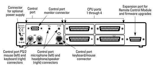
The ServSwitch Wizard DVI (4-port single-head model shown here) can support DVI video cards with up to four video outputs. They also support user stations with as many as four monitors.
