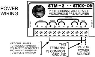
NOTE: THE STM-2 WILL OPERATE (WITH REDUCED HEADROOM) ON SUPPLY VOLTAGES FROM 9 VDC TO 23 VDC.
