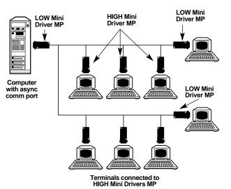
A two-line configuration is shown at right ("LOW" and "HIGH" are receive-impedance settings).
