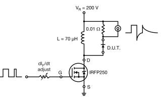
Fig. 9 - Reverse Recovery Parameter Test Circuit
